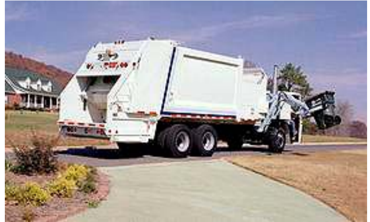
Rear – Loading & Side – Loading Truck with Automated Arm
